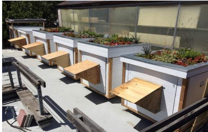
Figure 4: Green roof test cells
