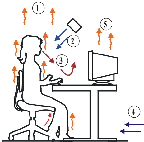
Figure 1. Personalized ventilation - Airflow interaction around human body: ① – free convection flow, ② – personalized flow, ③ – respiration flow, ④– ventilation flow, ⑤ – thermal flow
