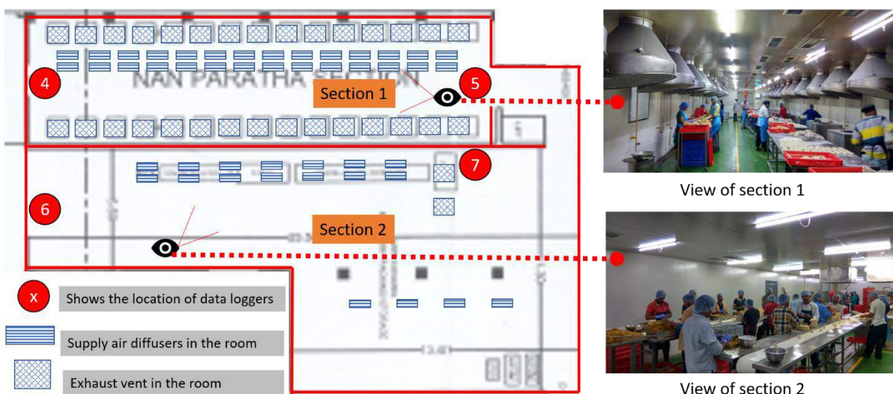
Figure 5 Plan showing data logger position, supply air and exhaust vents along with the view of both the sections
