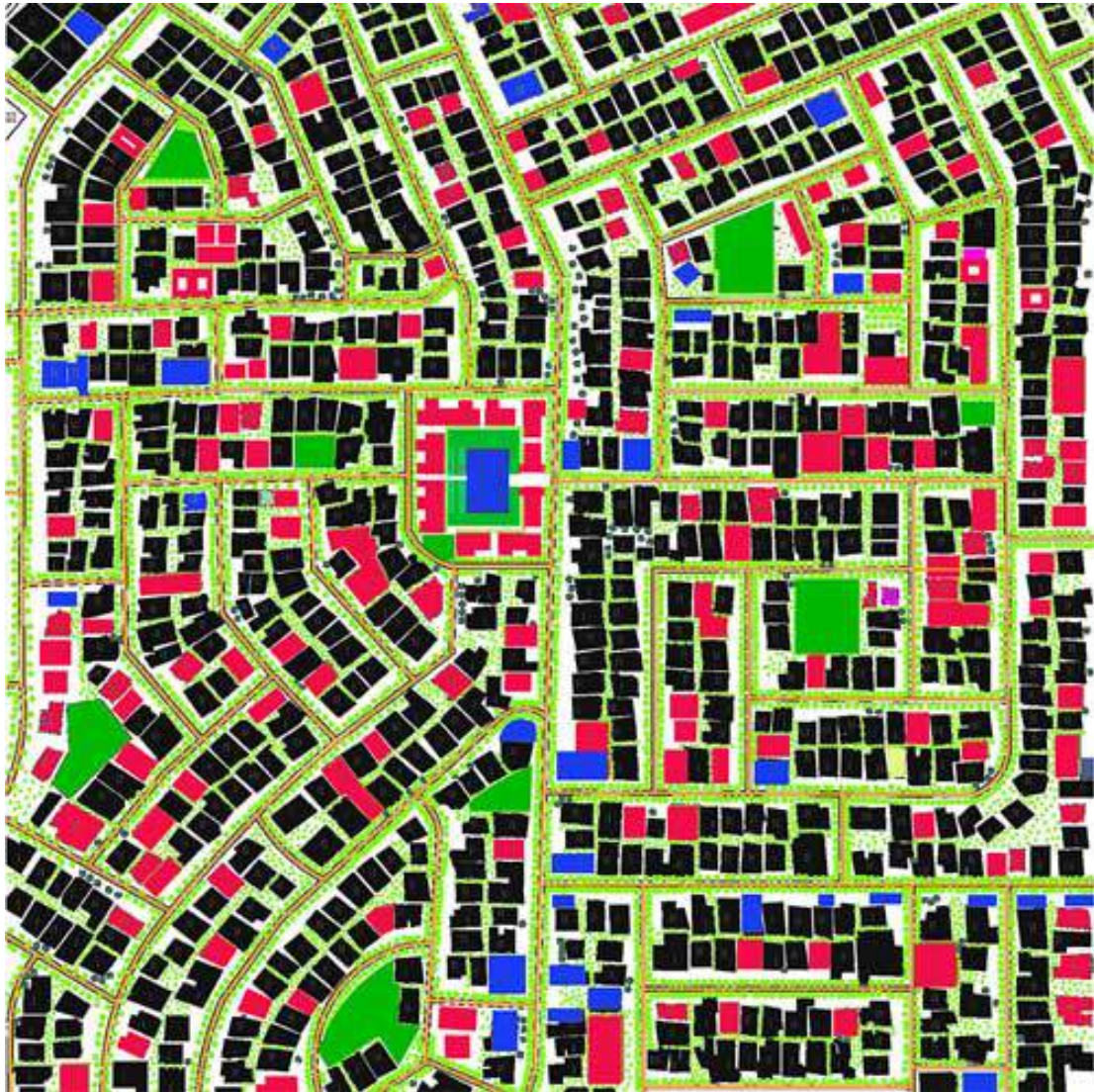
Figure 5. Enhancement proposal for the analysed residential area of 1 km 2 in Al Mawalih. Orange = pedestrian and bike network, black = existing buildings, blue = new public and commercial services, red = redensification with multistorey houses, green = recreational public spaces. (Source: Alexander Kader, 2018, based on design studios conducted with students from the German University of Technology in Oman)
