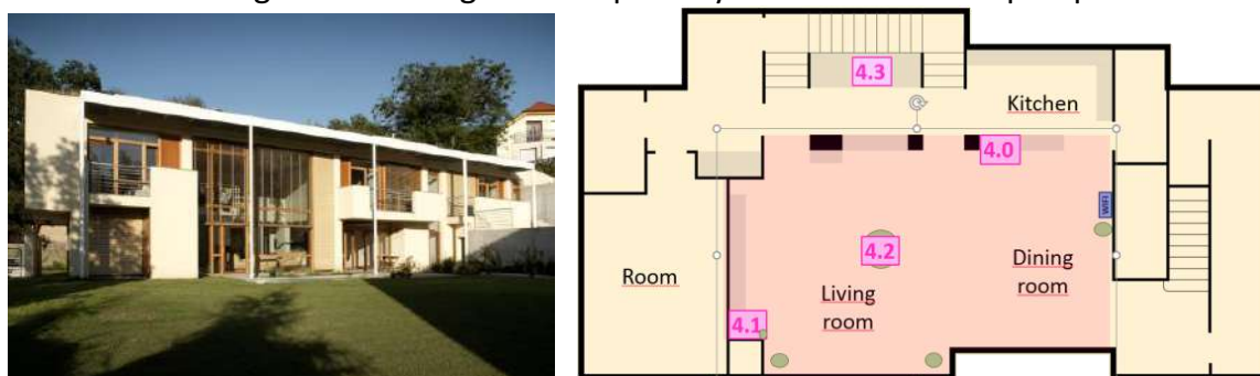
Figure 1 West view and ground floor of case study building with placing of measure points (4.0, 4.1., 4.2. a 4.3.)
