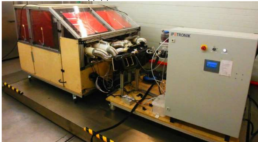
Figure 5. Simplified car cabin with supply platform (Wöhr, 2018, p. 36)
