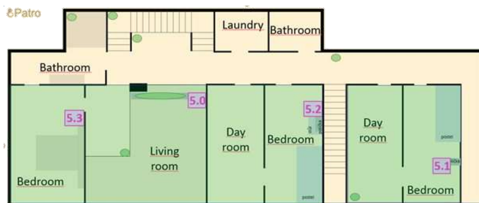
Figure 2 First floor of case study building with placing of measure points (5.0, 5.1., 5.2. a 5.3.)
