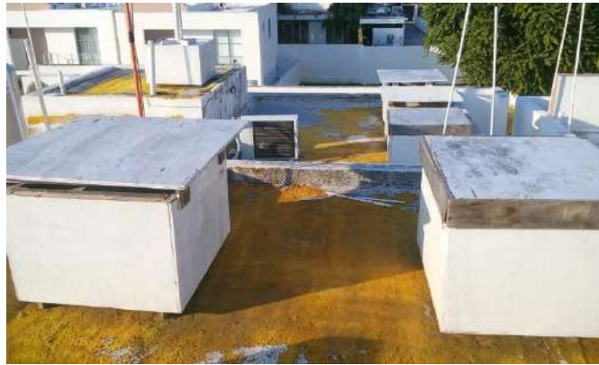
Figure 10. Experimental arrangement with during data monitoring of IEPCS complemented passive cooling techniques
