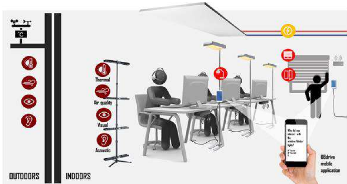
Figure 1. Simplified rendering of the eCOMBINE campaign used to inform occupants on the environmental, behavioural and energy monitoring (burgundy, red and yellow logos). Occupants are triggered to report comfort and motivation via desktop and app surveys.
