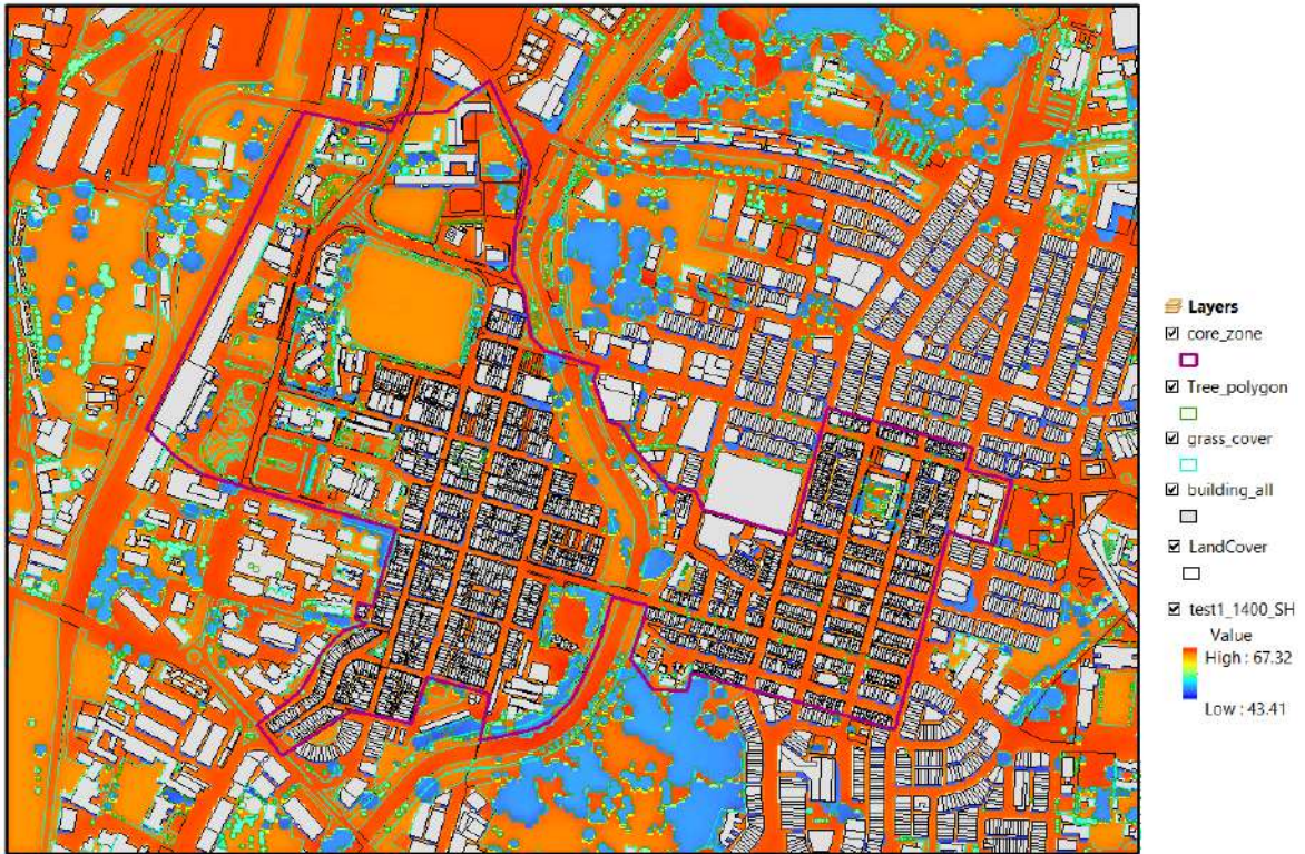
Figure 9. Mean radiant temperature distribution of 1400 LT at the height of 1.7m above the ground.
