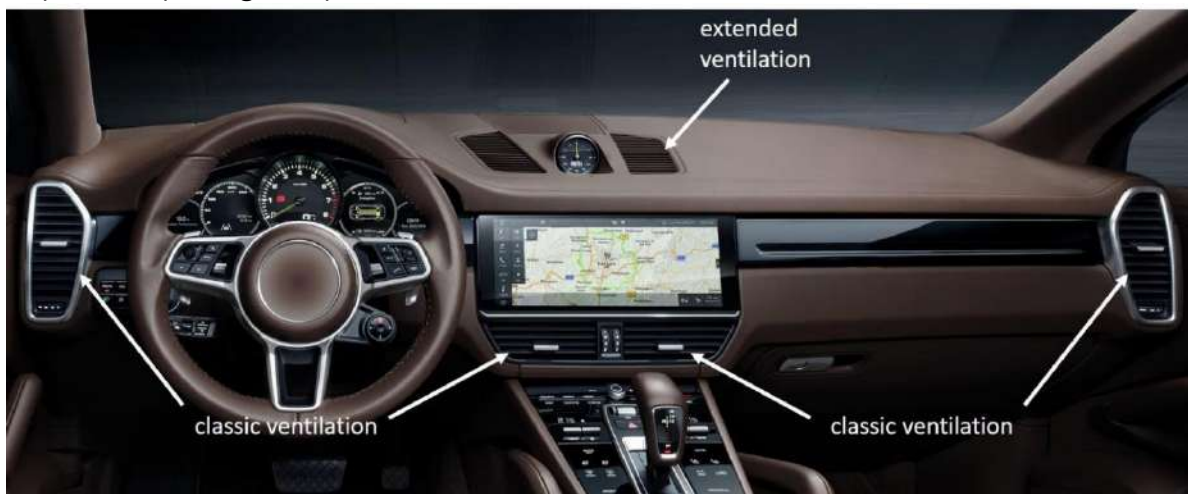
Figure 9. Standard air conditioning with EVF
