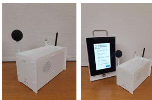
Figure 5. The indoor environment data logger (left); with the survey tablet (right)
