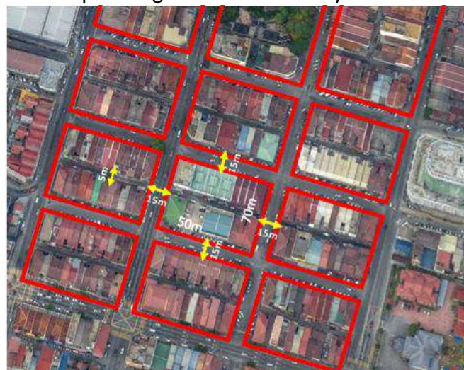
Figure 3. The characteristics of New Town in term of layout and pattern of building massing (adapted from: Google Earth, accessed 9 th July 2019).
