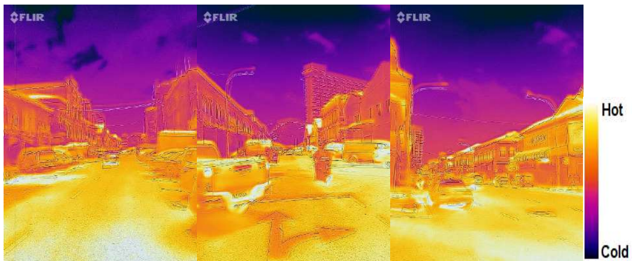
Figure 16. The surface temperature is highest at the typical asphalt roads with full concrete buildings and no greenery
